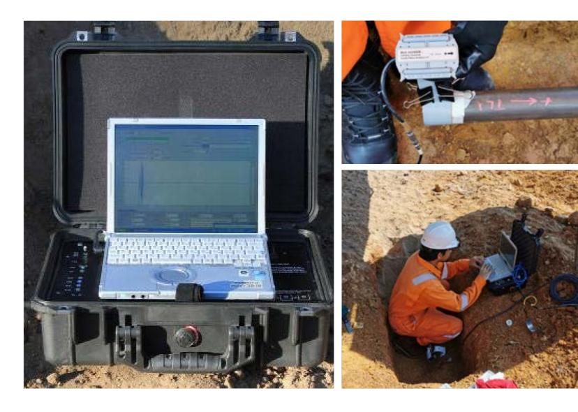
MsS System is a device that electromagnetically generates and receives low-frequency ultrasonic guided waves. It is used for rapidly surveying a long length of pipeline from a single test location. The corrosion wall loss and cracks in aboveground, buried, and insulated pipe can be detected, and their locations and sizes can be estimated by analyzing the data with user-friendly software.
